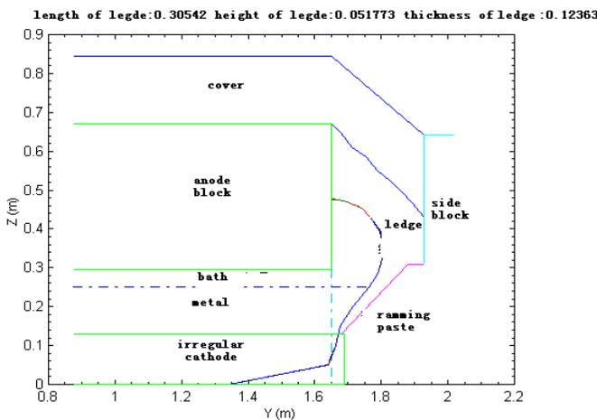
Figure 9. New thermal insulation lining structure, profile of pot side ledge
