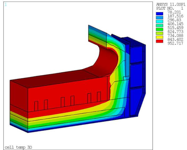
Figure 6. Conventional lining structure, pot end temperature
