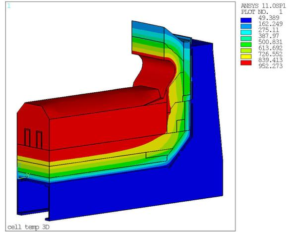
Figure 5. New thermal insulation lining structure, pot side temperature
